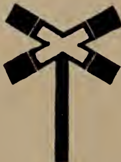
One track railroad crossing without gates
